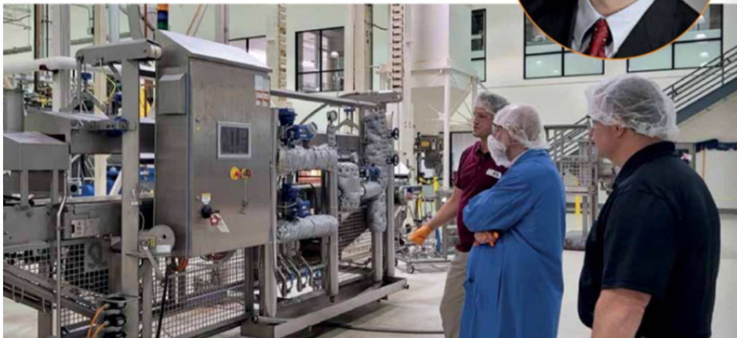
Jonathan Flowers, AFB Technician, showing how the Selo steam tunnel produces wet pet food and expands our capabilities to help customers trial new product concepts.
